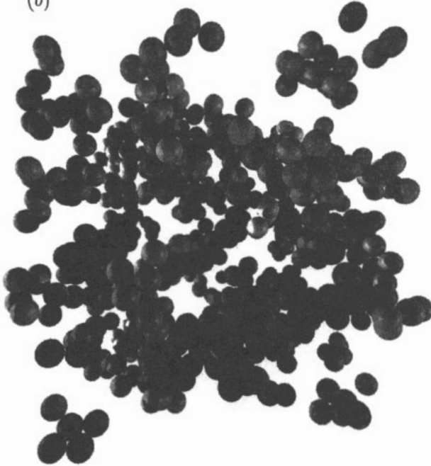
Figure 4. (a) The growth of the largest fractal cluster of connected nearest-neighbour droplets as a function of the volume fraction of the dispersed phase from 0.05 to 0.45. Snapshots taken from a Monte Carlo numerical simulation of the square-well potential with parameters a = 1.02 , \Delta = 0.02 , and \beta\epsilon = 3.7 , equivalent to Baxter's model with \tau = 0.1 . (b) A snapshot of the system, showing differently shaded nearest-neighbour clusters, at \tau = 0.1 and volume fraction of the dispersed phase 0.1.
